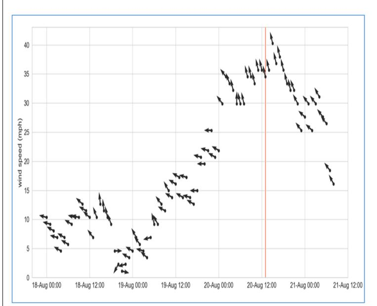
Wind speed and direction at Campbeltown before, during and after the incident at Carradale North. Circles denote wind speed. Arrows originating from circles denote wind direction. The orange vertical line denotes the approximate time of the incident.
