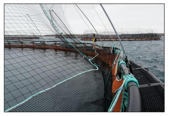
Figure 3: Image showing typical top-nets.
